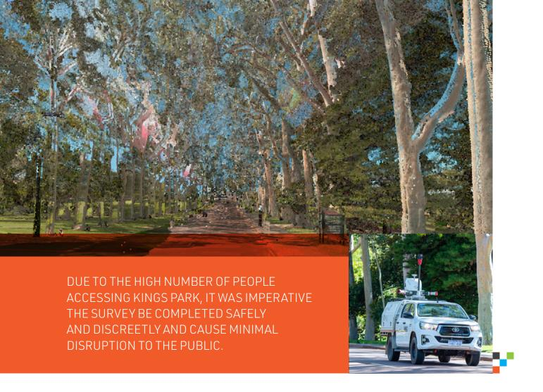
Utilising MLS meant the survey could be conducted without road closures and without active traffic management – helping keep people safe and minimise disruption. The dual scanner system provided high density data and, with multiple passes along the roadways, enabled a high-level of data analysis to maximise the accuracy of the survey.
